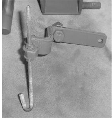
**Fig.6:Control arm (from front)**
